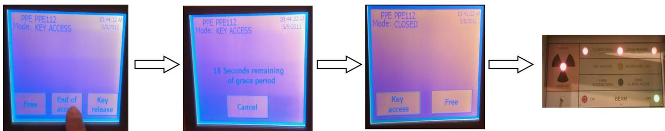
Using the CESAR beam terminal you can now switch the beam back on for the area.
